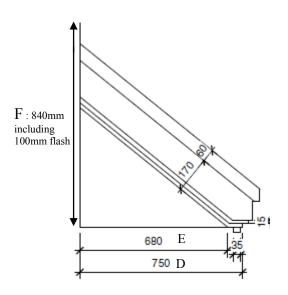
Front Elevation and side elevation
